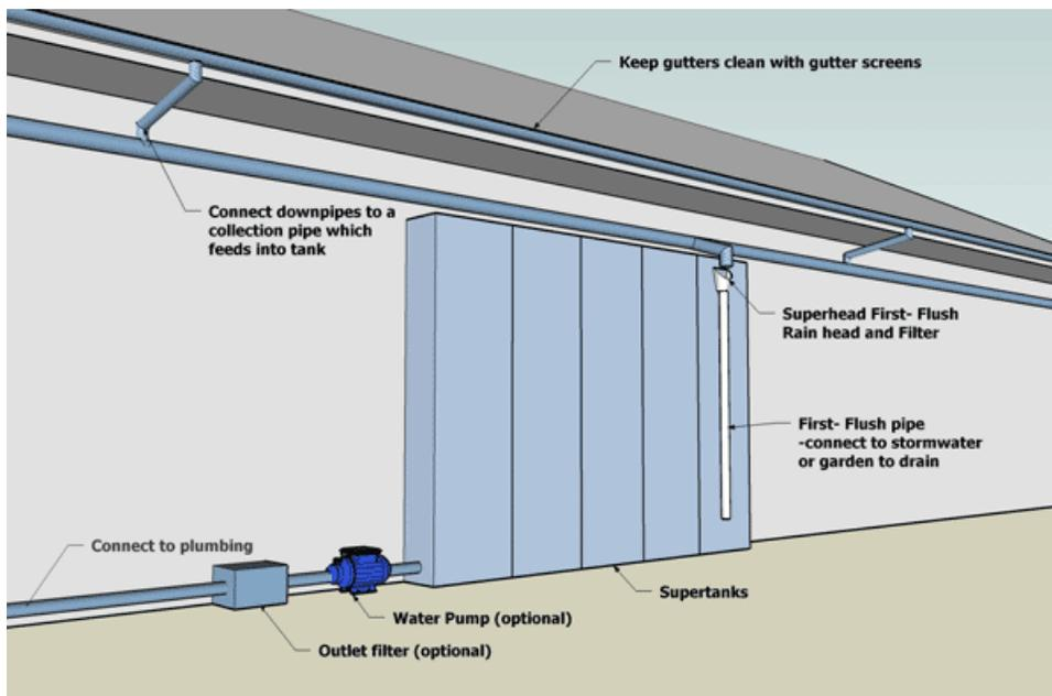
Example of the connections for a rainwater poly tank for capturing rainwater.
